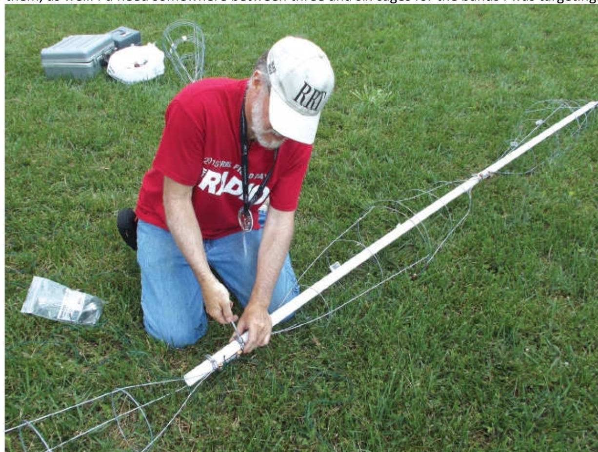
Figure 1 — The raw materials for the improvised 20 meter "Tomatopole" vertical consisted of several tomato plant cages made of galvanized wire, held together with split bolts; a bamboo stick for support; PVC pipe to keep it all upright, and a pair of 16-foot steel tape measures for radials.
