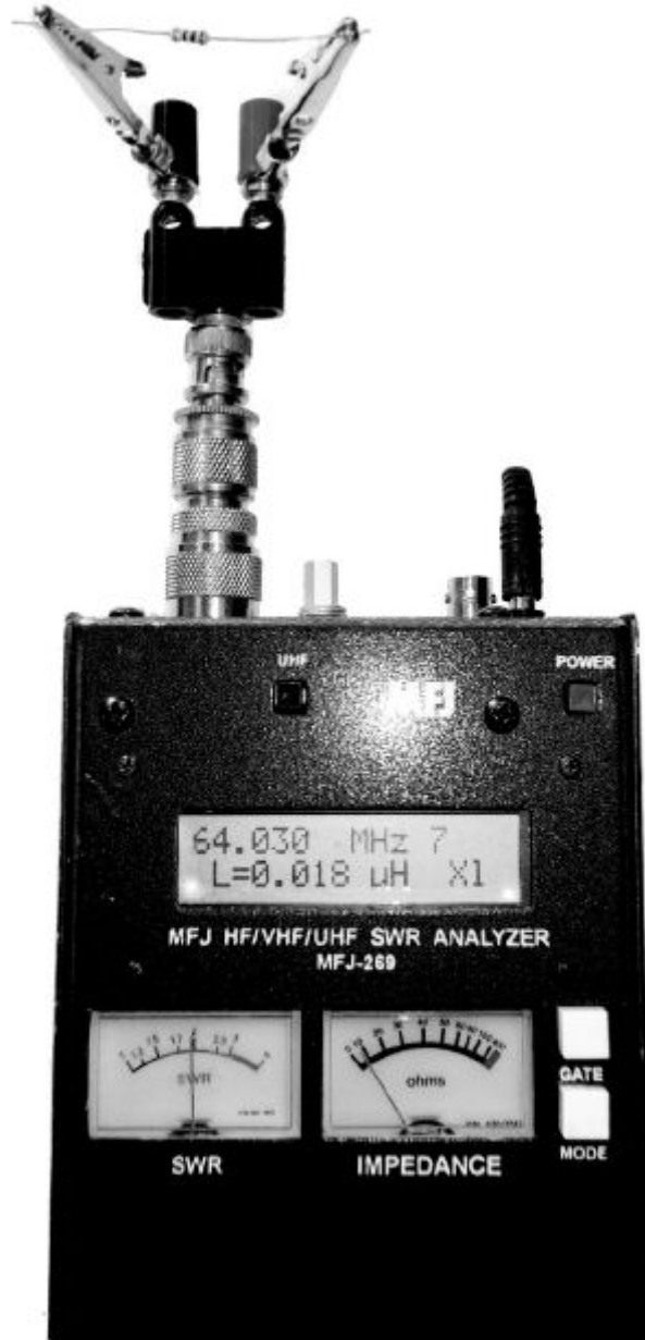
Figure 1 — A simple test fixture of alligator clips holding a 100 Ω resistor. The MFJ-269 antenna analyzer is showing an inductance of 18 nH (0.018 μH) at 64 MHz.
