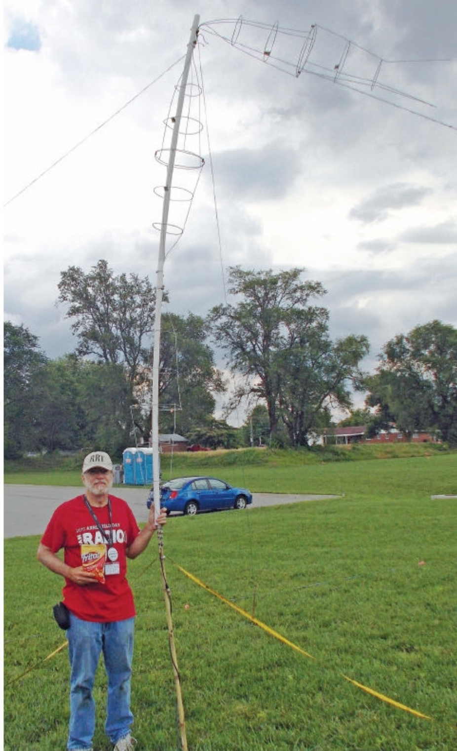
Figure 3 — Not bad for a little rummaging in the hardware store's garden department! The vertical resonated at 14.195 MHz with an SWR of 1.3:1 and made plenty of contacts. The Fritos are optional.
