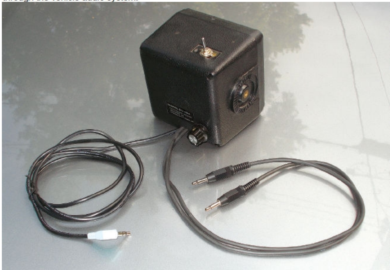
Figure 4 — The completed speaker with the volume control, on-off switch, and cables for connection to the radios and vehicle audio system (white connector). [Ward Silver, N0AX photo]
