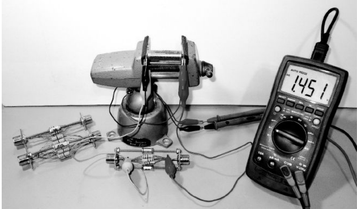
Figure 1 — The test setup for battery load tests. Loads are constructed from multiple resistors in parallel. The battery is held between two copper pennies in a vise with insulating jaws. Clip leads are used to connect the battery, load and logging DMM.
