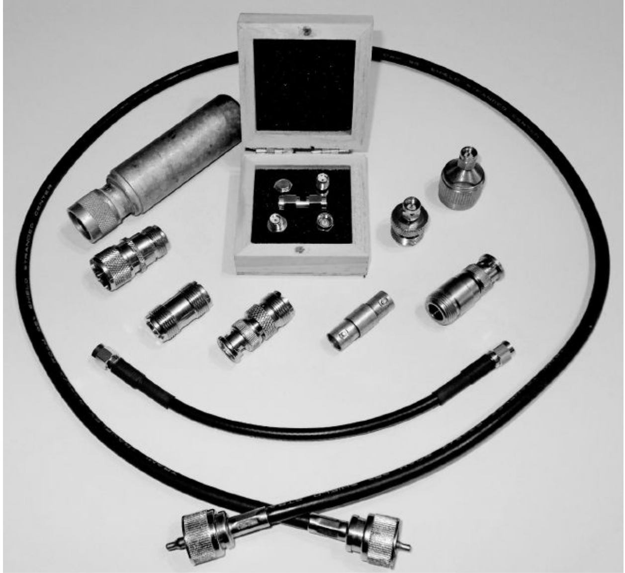
Figure 1 — A set of calibrated SMA-series loads in the small box include a short, open, and 50\ \Omega , along with double-female and double-male adapters. The 5 W 50\ \Omega dummy load is flat (non-reactive) to well over 1 GHz. A set of coaxial adapters includes cross-family and double-female adaptors for UHF, N, BNC, and SMA connectors. The pair of jumper cables completes the package.
