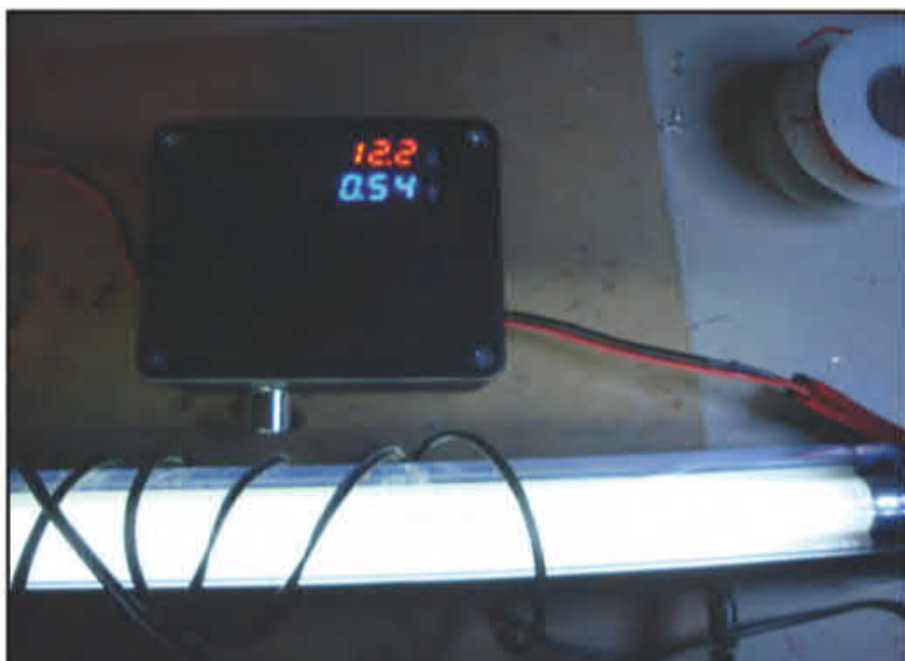
Photo H. Final test — setting the output to operate a 12-volt fluorescent lamp.
