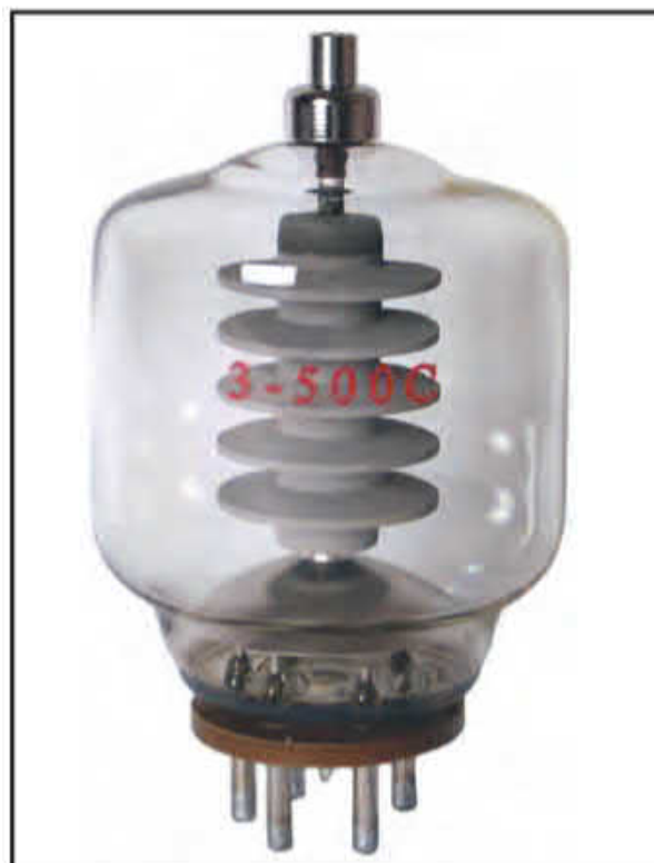
Photo D. A 3-500 C vacuum tube used in many HF amplifiers today.
