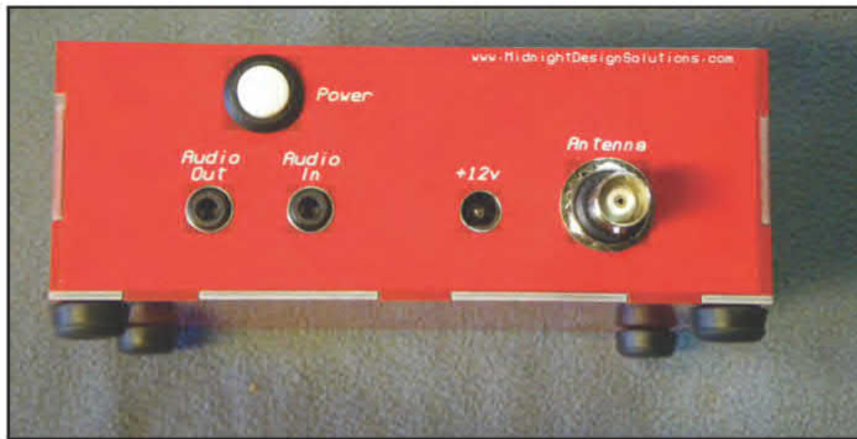
Photo D. Rear panel of the Phaser enclosure. It is made from PC board material. Note the notches on the bottom and sides that help the pieces fit together more precisely.
