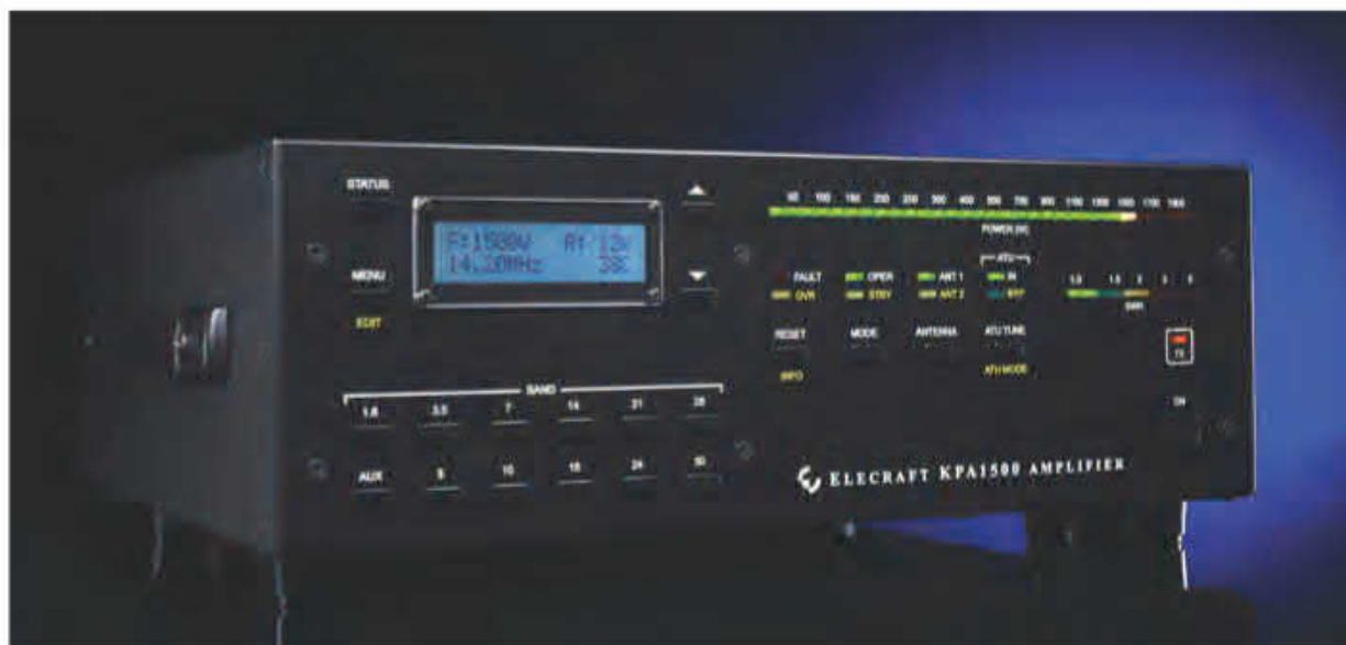
Photo E. Elecraft's new solid-state KPA 1500 HF amplifier. Like many solid-state amplifiers, it requires no manual tuning and it can deliver full, legal limit power output. (Photo from Elecraft website)
