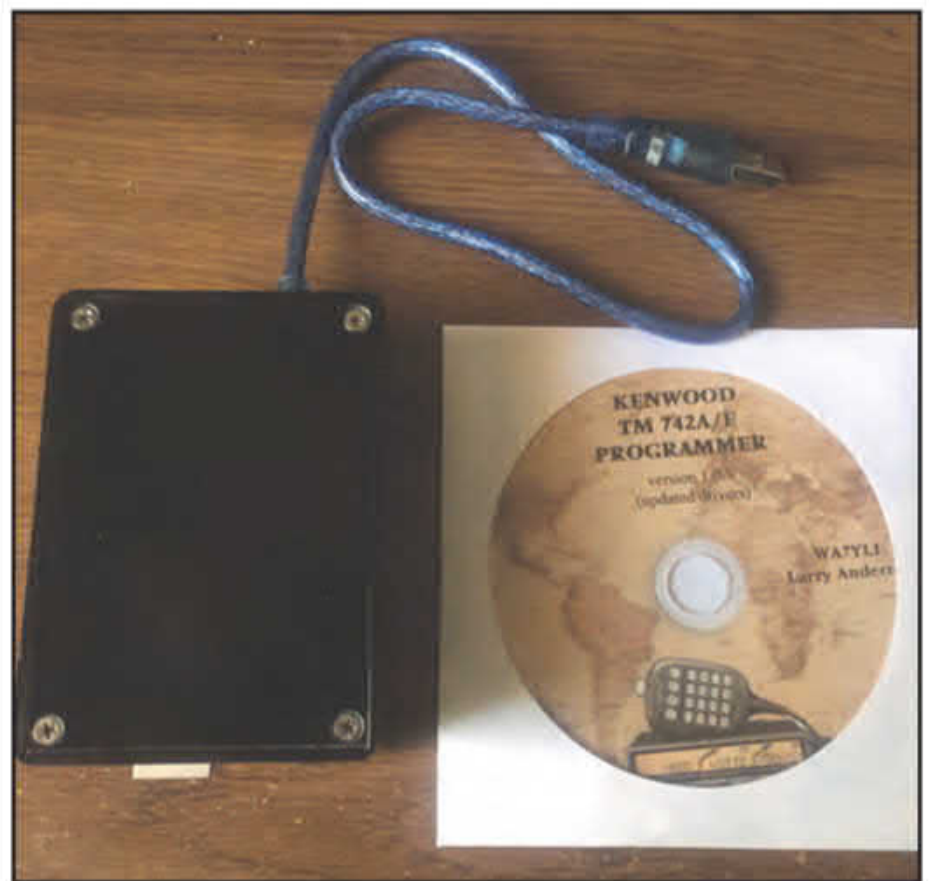
The TM-742A/E programming kit from WA7YLI brings some much-needed memory management utility to Kenwood's vintage triband transceiver.
