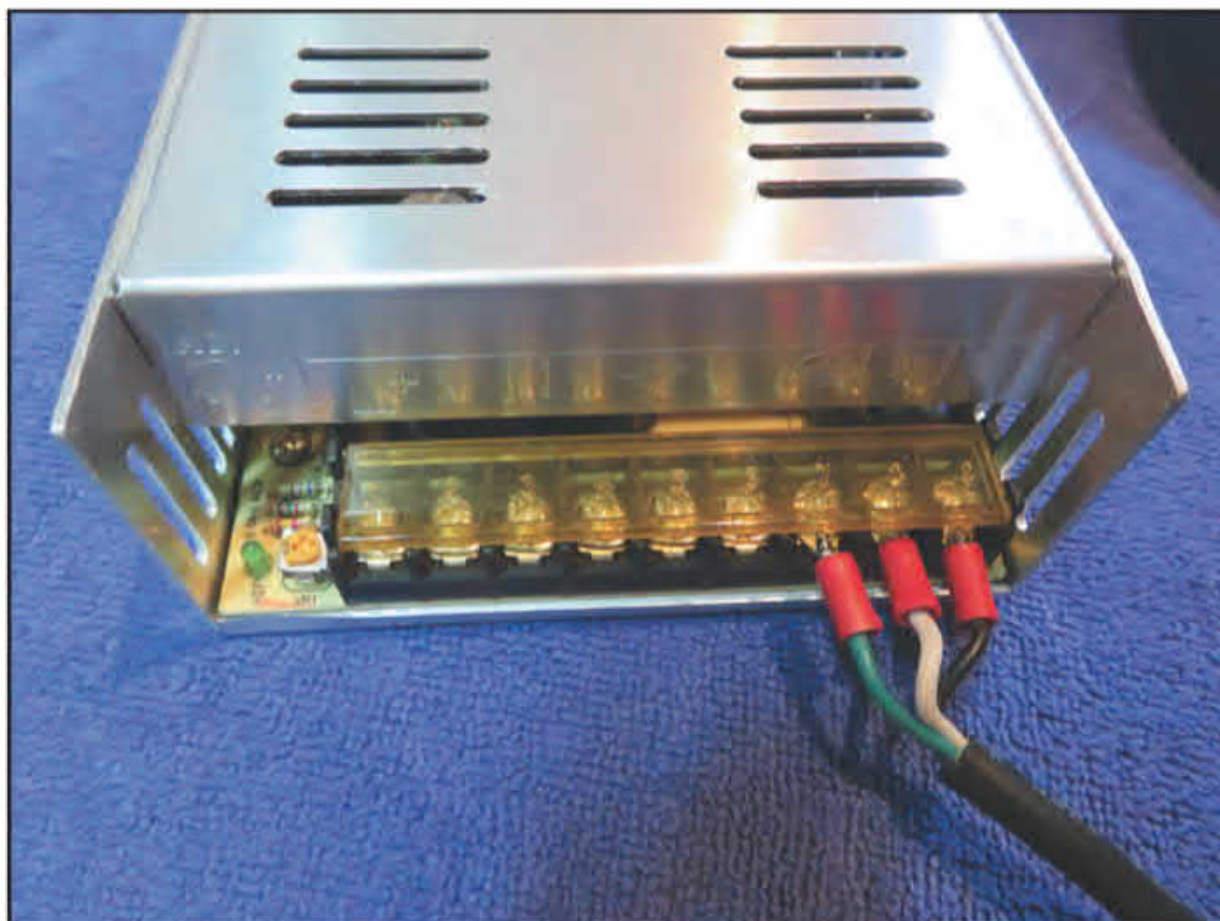
Photo C. The end terminal strip is marked, showing the AC input and the DC output terminals. The trimpot on the left adjusts the output voltage.
