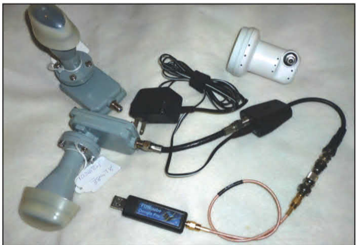
Photo D. Low-cost 10.45-GHz system for receiving 10.45-GHz AMSAT satellite downlinks.
