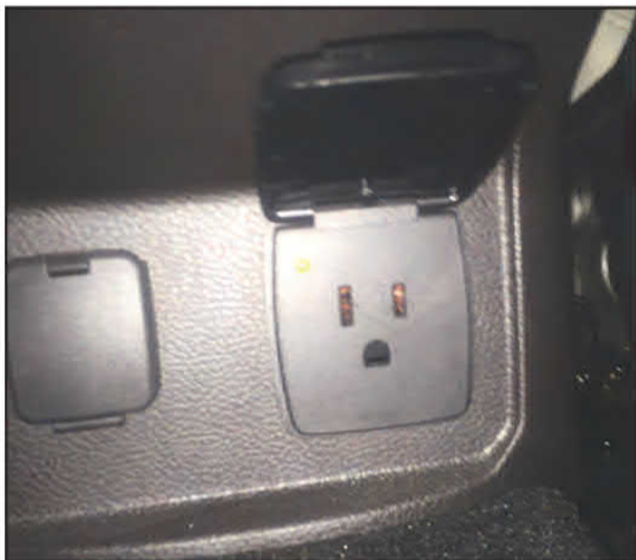
A 110-volt outlet found in the back seat of the author's 2016 Ford Fusion. A 12-volt port is located to the left.
