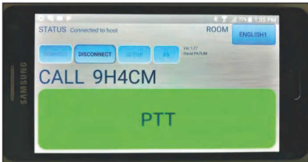
Photo A. An Android phone using the Peanut app. As shown, it is in the receive mode.
