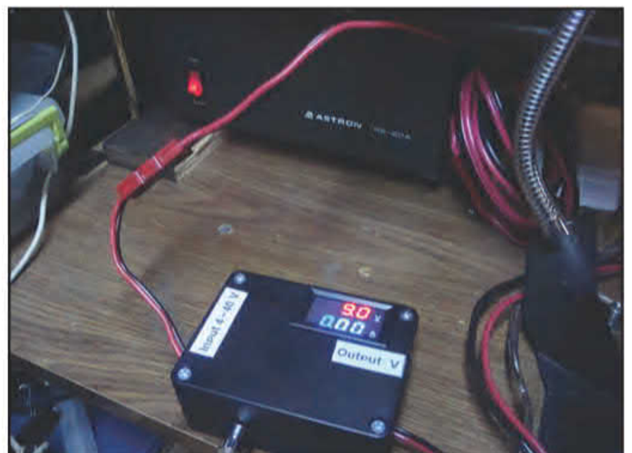
Photo I. Astron power supply and adjustable converter set to about 9 volts.
