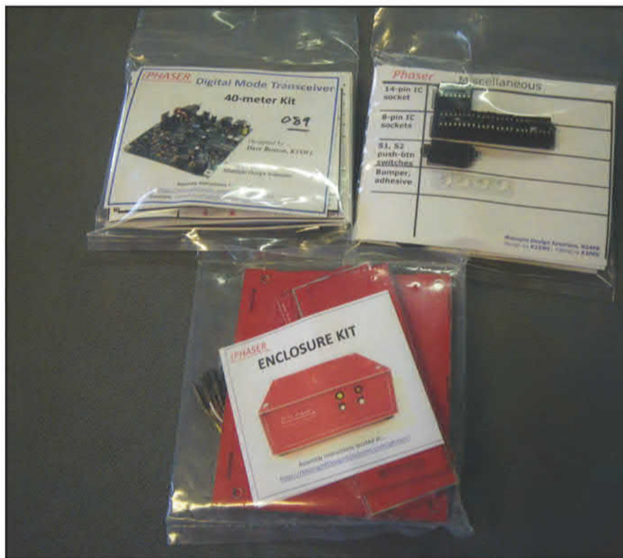
Photo A. The Phaser transceiver kit came packed in three bags, two for the radio and one for the optional enclosure kit. Note the “parts card” in the package on the upper right to which various components are attached after sorting. (Photos / illustrations by the author)
