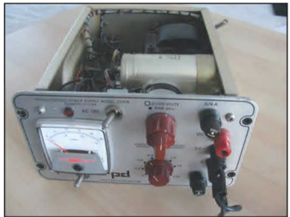
Photo C. This old variable power supply will get a new power cord, new electrolytic capacitors, and possibly other components.
