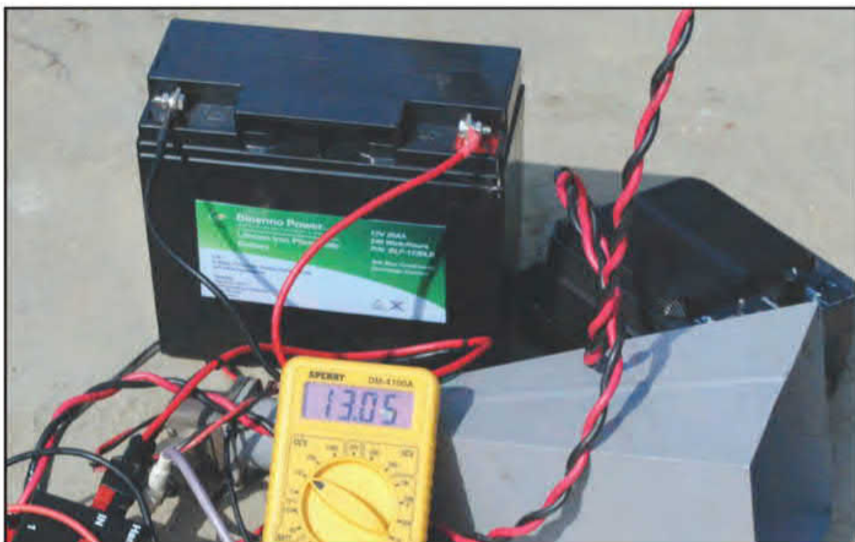
I use the 12 amp-hour (Ah) LiFePO4 battery during a day of microwave contacts.
