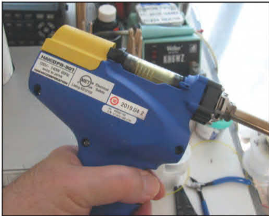
Photo A. My new desoldering iron makes repairing and harvesting parts easy and fast.
