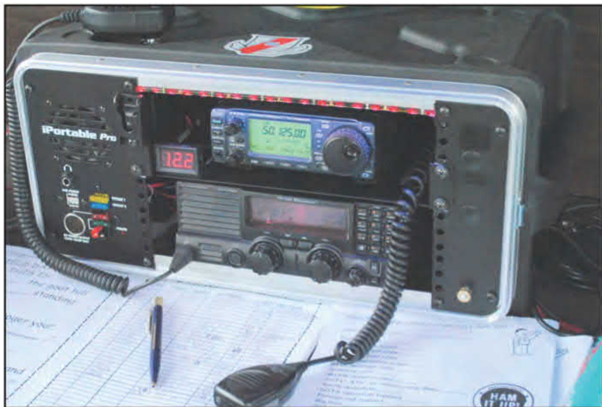
My HF radios ran on the internal 20-Ah LiFePO4 battery for a weekend, with 12 volts still to spare!
