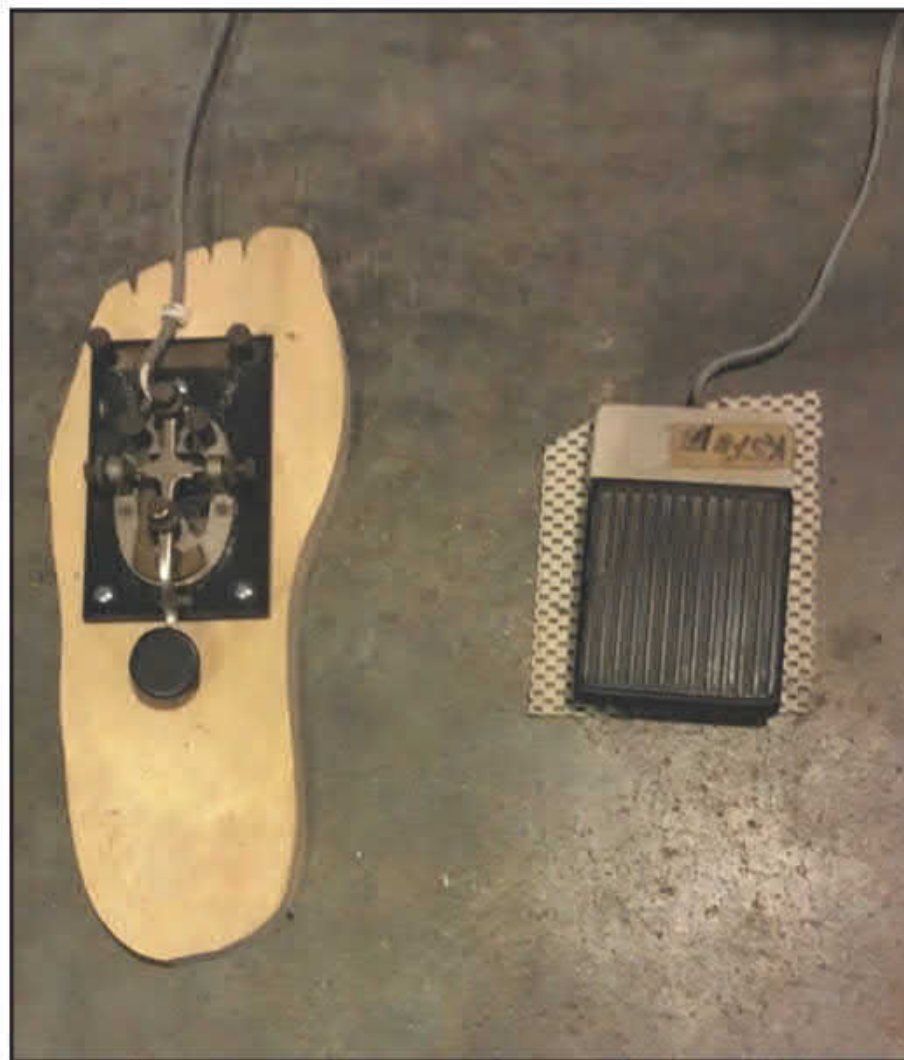
Photo A. The footswitch allows hands-free operation. It can be simple or elaborate. The one on the left uses an old hand key mounted to a board. It's also handy for QLF contests. 2 The one on the right comes from a yard sale.
