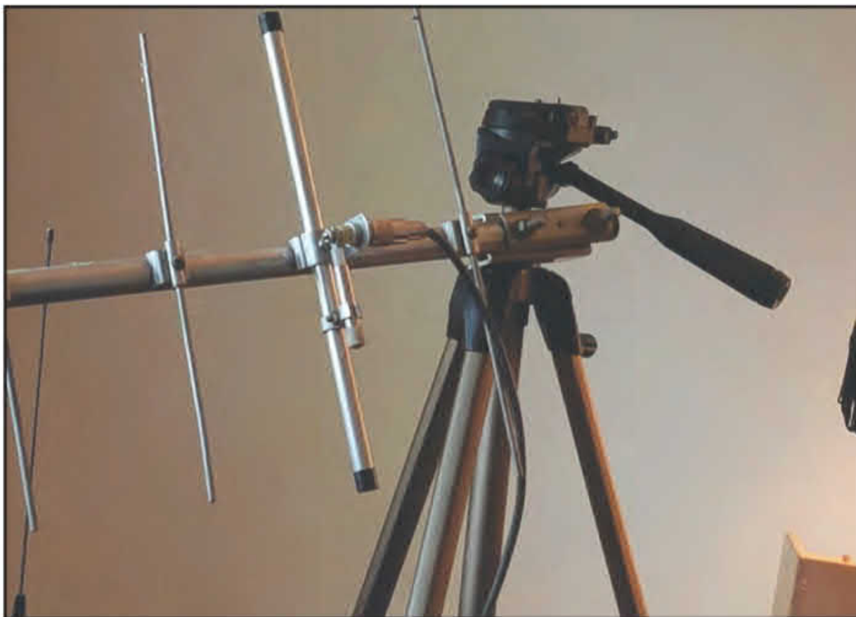
Photo A. A 70-centimeter, gamma-matching network on a small Yagi antenna. Matching networks introduce some losses. (All photos by KOØZ)
