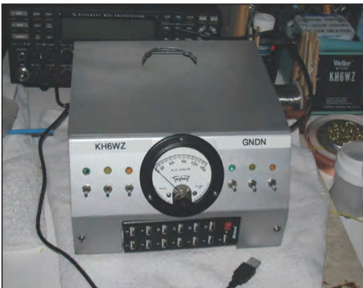
Photo L. A desktop "Goes Nowhere, Does Nothing" box. It does have a powered USB hub and fan. The meter serves as a power-on indicator.
