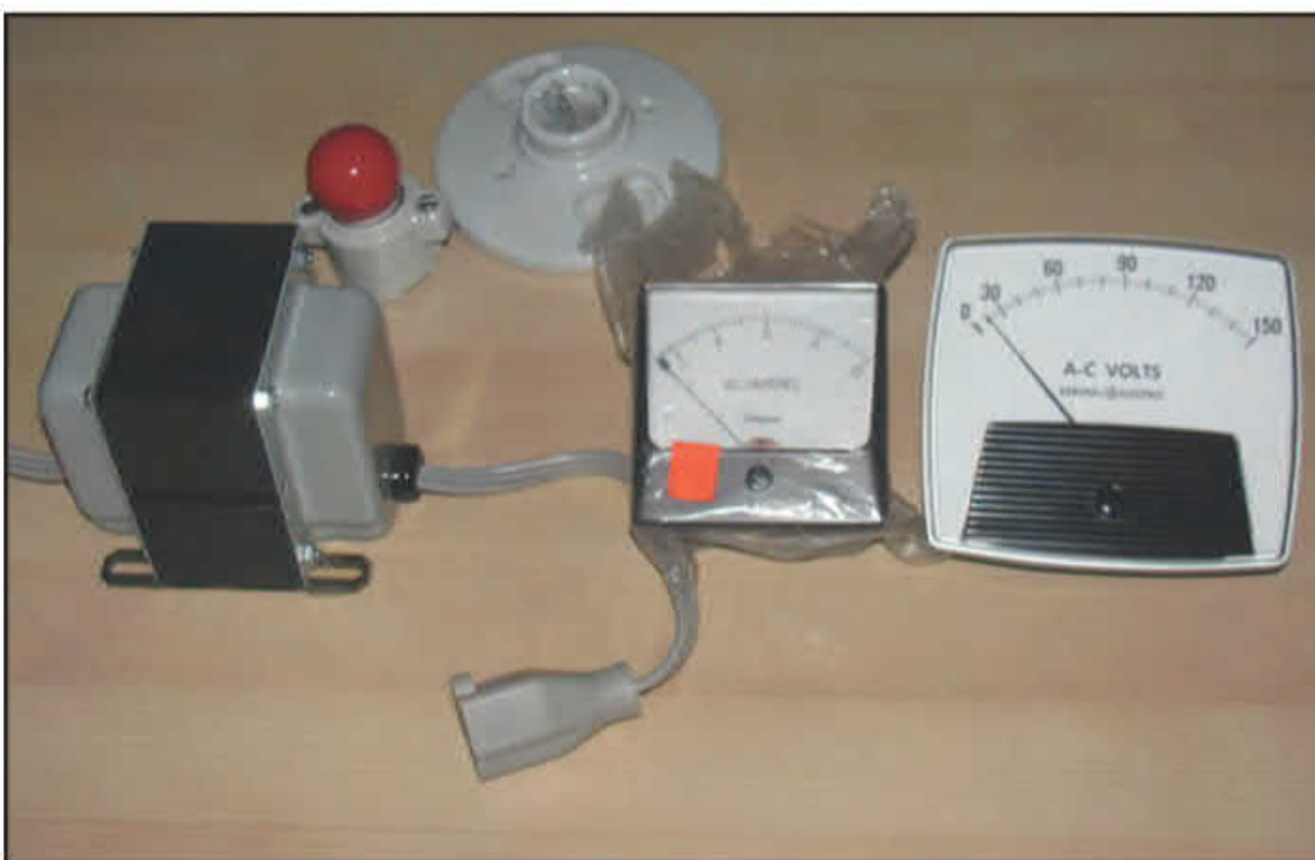
Photo F. These parts from my junk box will become an isolated, variable AC power supply. It will ensure safe testing of unknown power transformers and other AC line-operated devices.
