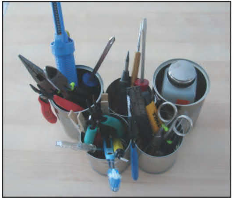
Photo B. This bench-top tool caddy got its inspiration from a book by Adam Savage. The simple idea makes selecting a particular tool fast and easy. To build it, I used empty tin cans that are grouped and held together with hot glue.
