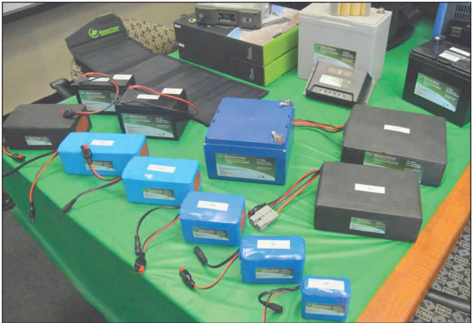
Lithium iron phosphate (LiFePO4) batteries offer more energy and half the weight compared with traditional lead-acid batteries.
