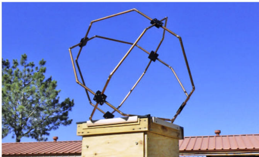
Figure 4 — U.S. Navy HF vector-sensor array [Source: J.H. Meloling, et al., 2016].
