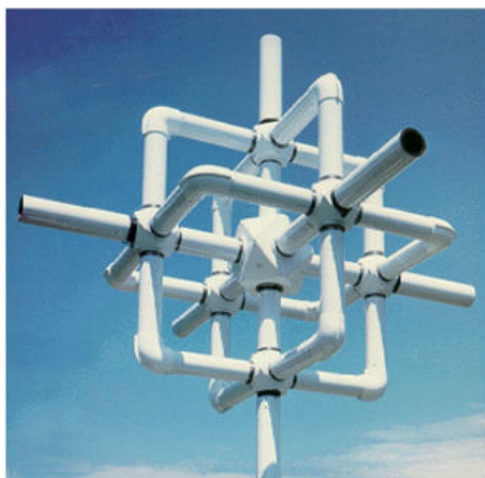
Figure 2 — Flam & Russell SuperCART array [Source: Bull and L.R. Burgess, 1990].
