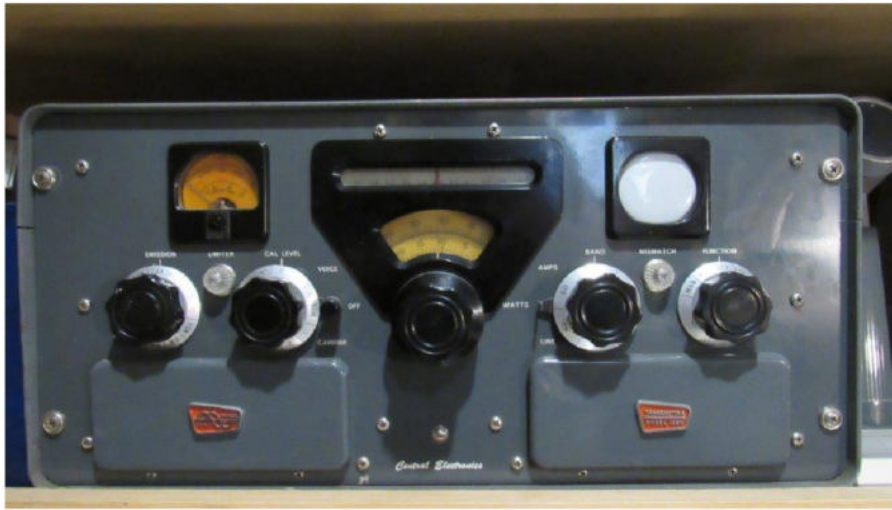
Figure 3 — The Central Electronics 100V transmitter uses two double balanced mixers in quadrature to generate a wide range of modulations.
